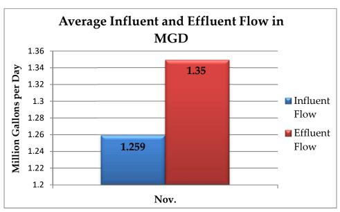
This graph represents the average daily flow into the treatment plant as well as the average daily flow discharged into the Kinnickinnic River. The design flow for the Treatment plant is 1.8 million gallons per day (MGD).
