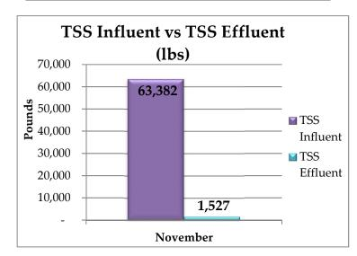
The TSS Influent and TSS Effluent represent the pounds of Total Suspended Solids entering the Waste Water Treatment Plant versus going out into the Kinnickinnic River.
